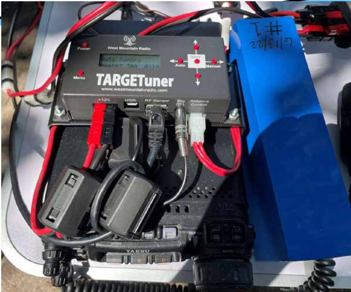
Yaesu FT-857D with Target attached to radio bracket, connected per instructions. Note: I am sure I used more ferrites than necessary.
