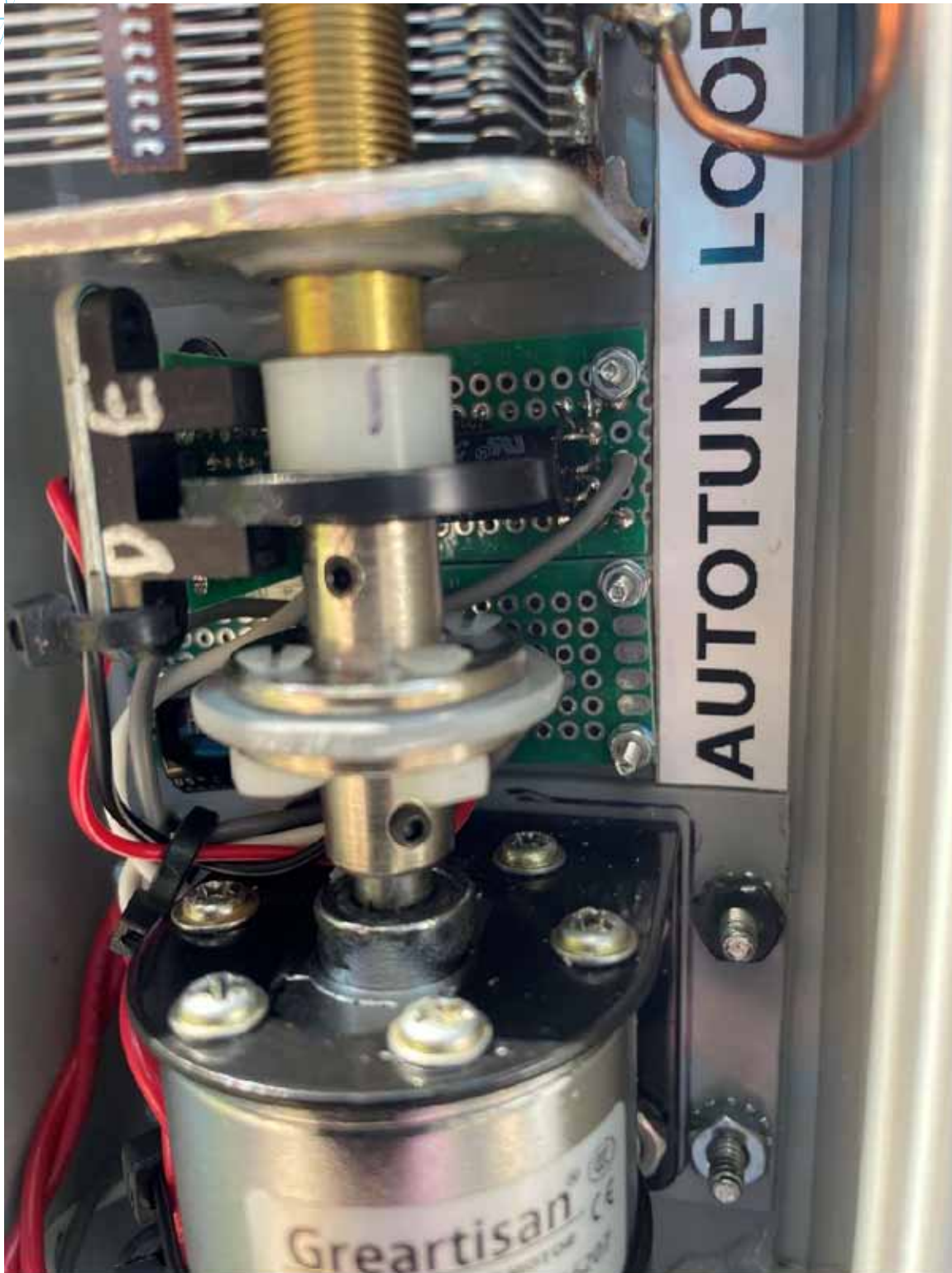
Opto-Interrupter layout Detail, Enclosure was closed to prevent light from interfering with pulse count.
