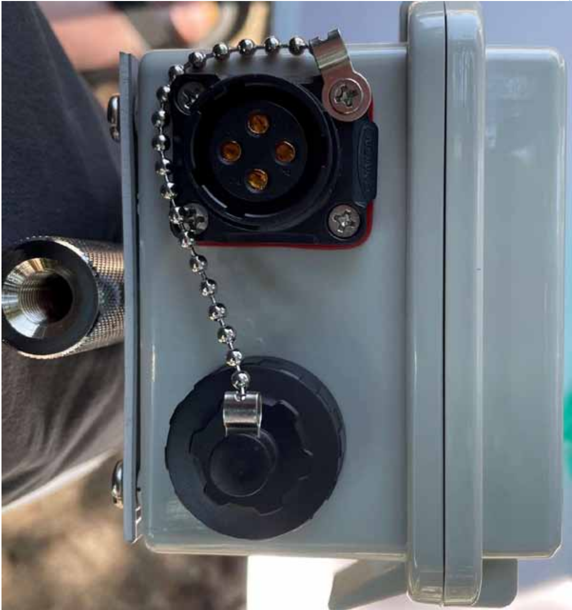
4 pin connector detail with dust cap off. Enclosure is mounted on a sub-plate with four screws to cut down on the number of holes put in the box. Mast mount assembly bolted to plate with brackets.
