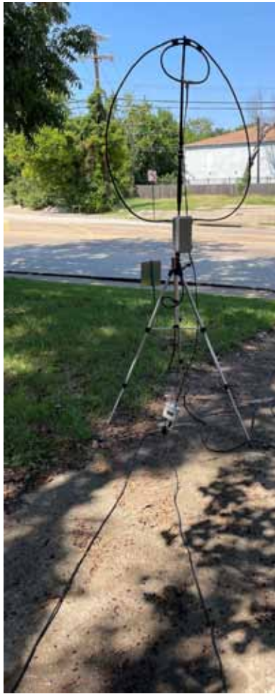
Alpha Loop showing cables separated from each other.
